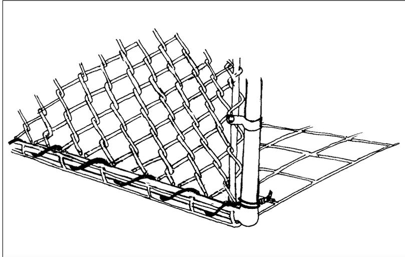
*Garden fencing wired to upright chain link panel using the "sewing technique"*
